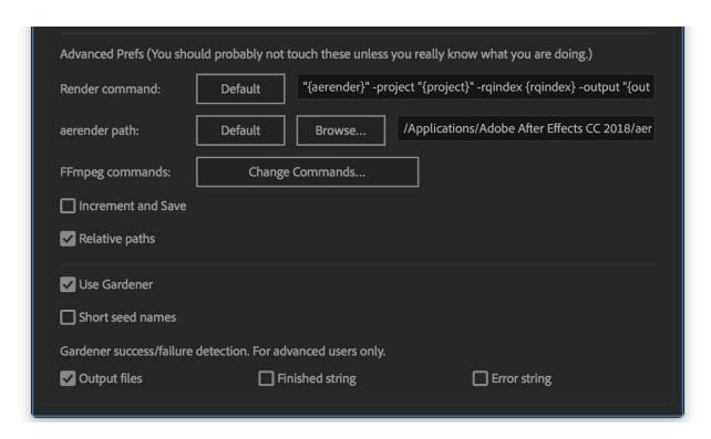
Render Command: This is the command sent to aerender to submit the comp. We include a number of flags which are needed for consistent renders. Power users can modify the flags in this text field, but in general this should not be modified. If anything goes wrong with your changes you can always hit the "Default" button to return to the factory settings.
